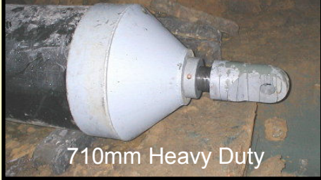
Hollow stem with 1 way valve for ballasting
